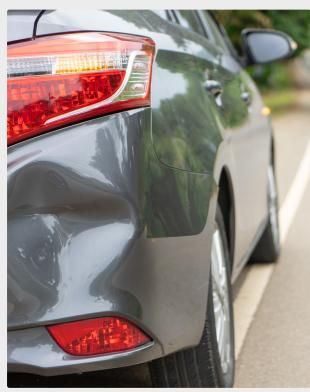
Paintless Dent Repair provides an innovative process to remove small dings and dents from painted surfaces without harming the vehicles factory finish.
