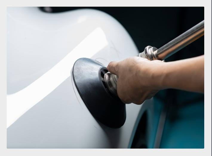
Using special tools and techniques developed by auto manufacturing teams, technicians are able to permanently remove door dings and minor dents.
